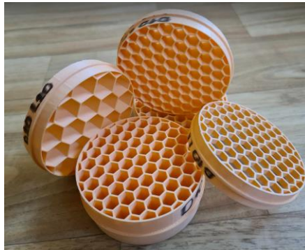
Fig.1. Stream honeycomb straighteners used in the experiment
